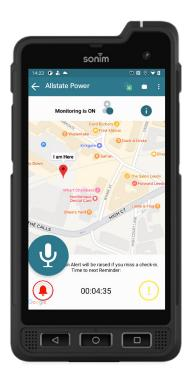
As well as tracking the location of users, our keep alive enables employees to be periodically checked, in real time, either directly, via the application, or by detecting their behaviour using sensors on the device. These include if the device tilts, or is shaken or dropped, to detect falls. No movement/device inactivity or high speed can also be detected.
